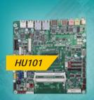
4th Gen Intel® Core™ U-series Processors 2 DDR3L SODIMM up to 16GB 1 LVDS/eDP, 2 HDMI 2 GbE, 4 COM, 10 USB 1 PCle x1, 1 Mini PCle
