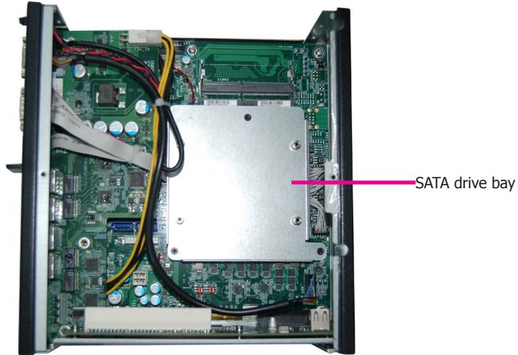
2. Insert the SATA drive into the HDD bracket and secure it in place with the provided screws (black screws). The HDD bracket can accommodate two SATA drives.
