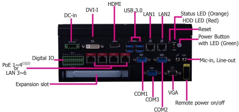
The front panel I/O consists of the following ports from the mainboard:
