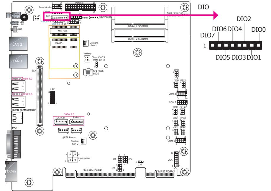
The Digital I/O connector provides 8 digital input or output port to enable monitor and control of the states of the connected external devices. Note that the HW Utility can only configure the external DIO ports. Please see “Digital I/O Connector (daughter board)” in this chapter.
