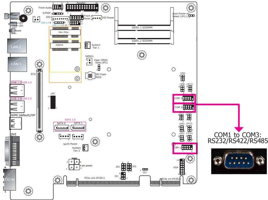
COM1 to COM3 can be selected among RS232, RS422 and RS485 via jumper settings. In addition, COM1 and COM2 can be switched between normal RS232 and RS232 with power. For pin definitions and jumper selection for different communication modes, please refer to Chapter 4. The serial ports are asynchronous communication ports with 16C550A-compatible UARTs that can be used with modems, serial printers, remote display terminals, and other serial devices.
