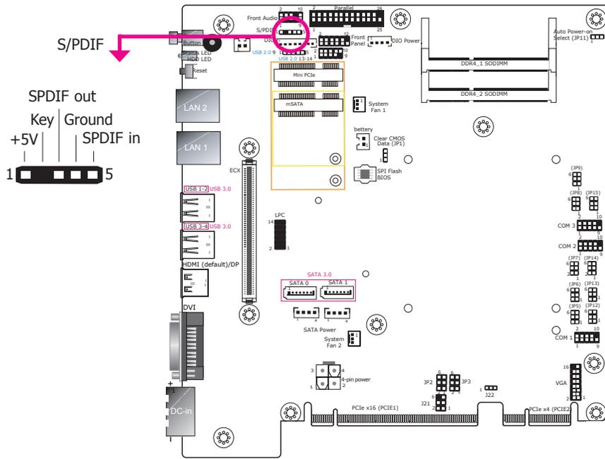
The S/PDIF connector is an audio interface for transmitting digital audio signals. The system includes an S/PDIF header on the mainboard. Make sure pin 1 of the audio cable is aligned with pin 1 of the S/PDIF connector.
