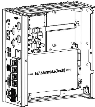
1. The PCI and PCIe slots on the riser card inside the system are used to install expansion cards. To install an expansion card you need to first remove the slot plate and bracket by uninstalling the screw on the front chassis.
