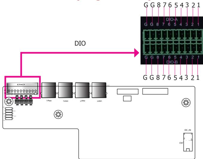
The Digital I/O connector provides 16 digital inputs or outputs to enable monitor and control of the state of the connected external devices. You can use the provided HW Utility to configure a port to be either input or output. Please refer to Chapter 8 for more information.
