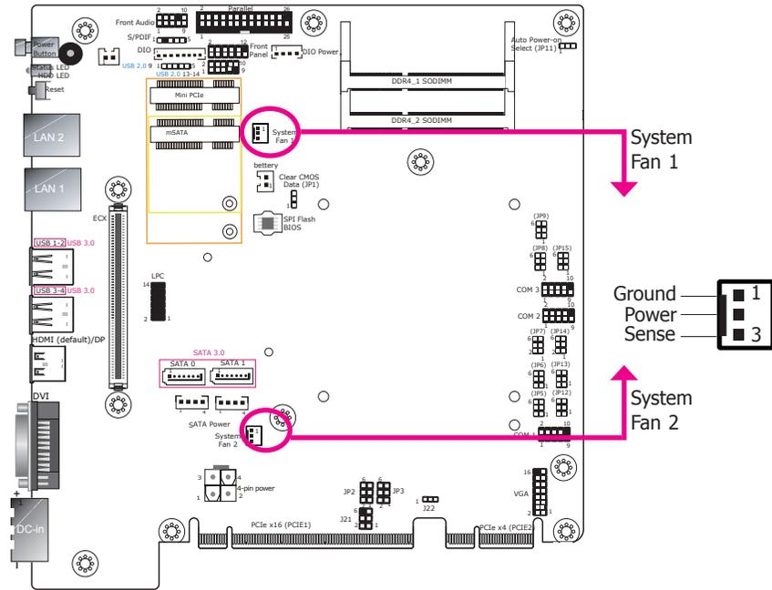
The fan connectors are used to connect cooling fans.
