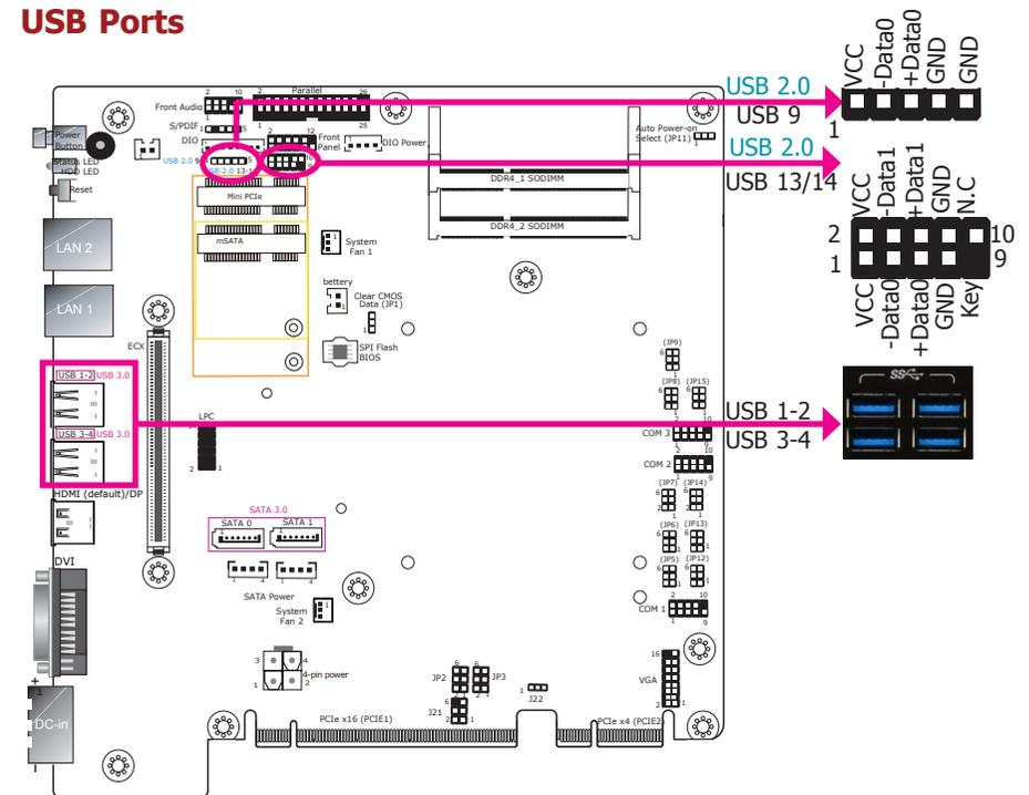
The USB device allows data exchange between your computer and a wide range of simultaneously accessible external Plug and Play peripherals. In addition to the 4 external ports on the front panel, the system board provides 3 USB 2.0 ports through internal pin headers.
