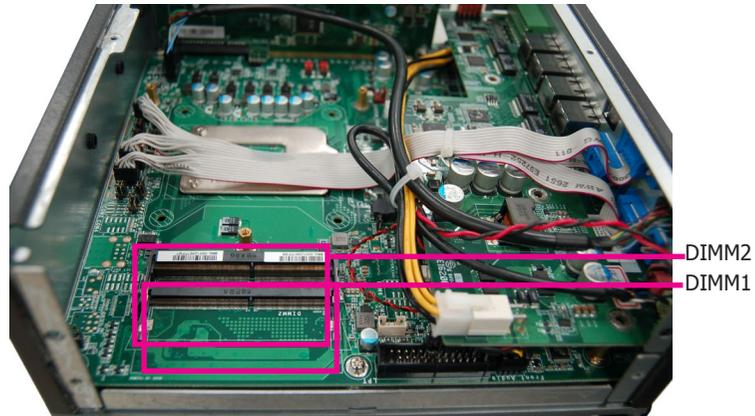
To remove a SODIMM, gently spread the retaining clips at each end of the SODIMM socket. The SODIMM should pop out of the socket. Lift the SODIMM away from the socket on the mainboard.
