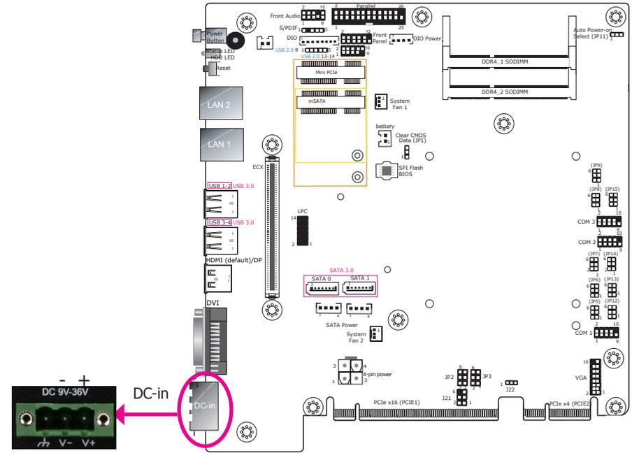
This three-terminal block connector provides options of power input solution: 100W, 120W, and 160W. Connect a DC power cord to this jack. Using a voltage higher than the recommended one may fail to boot the system or cause damage to the mainboard.
