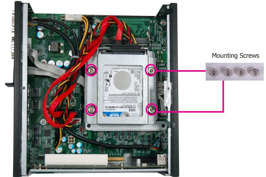
4. Connect the other end of the SATA data cable and the SATA power cable to the SATA data and SATA power connector on the mainboard respectively.
