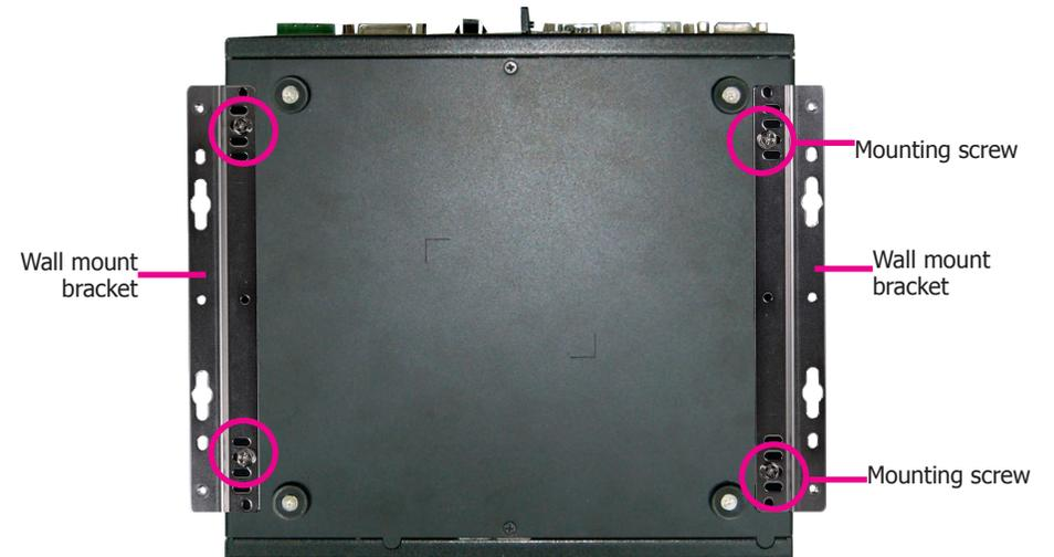
The following illustration shows the location and dimension of the holes for mounting the device onto a wall or rack .
