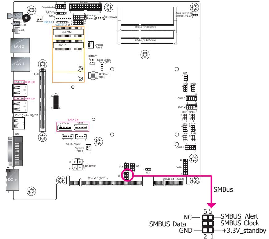
The SMBus (System Management Bus) connector is used to connect SMBus devices. It is a multiple device bus that allows multiple chips to connect to the same bus and enable each one to act as a master by initiating data transfer.
