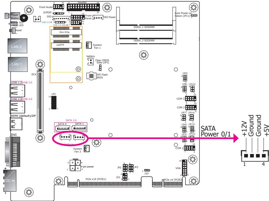
These SATA power connectors supply power to SATA drives. Connect one end of the provided power cable to the SATA power connector and the other end to your storage device.
