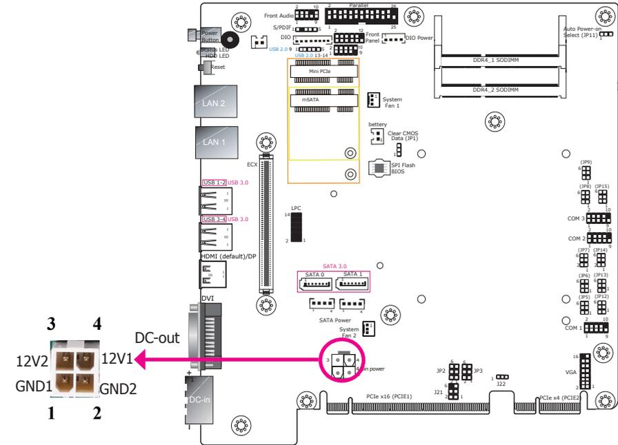
The 4-pin vertical type connector (optional) provides low power output.
