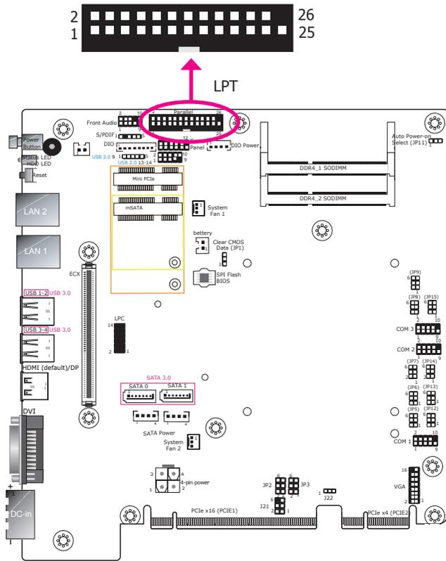
The 25-pin connector is used to connect the parallel port of a device such as a printer. It supports SPP, ECP and EPP standards.
