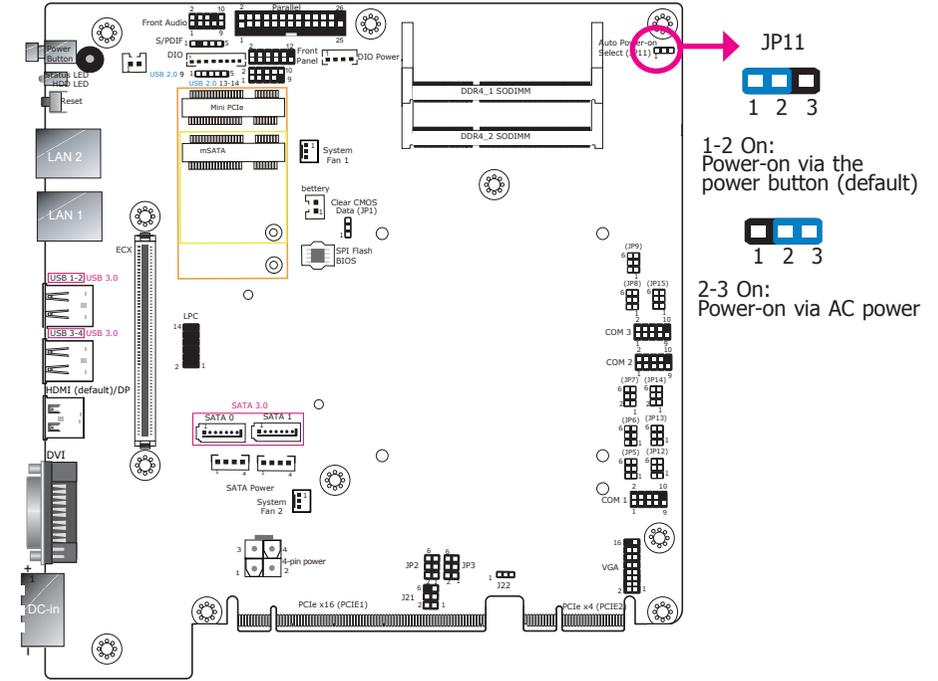
JP11 is used to select the method of powering on the system. If you want the system to power-on whenever AC power comes in, set JP11 pins 2 and 3 to On. If you want to use the power button, set pins 1 and 2 to On.
