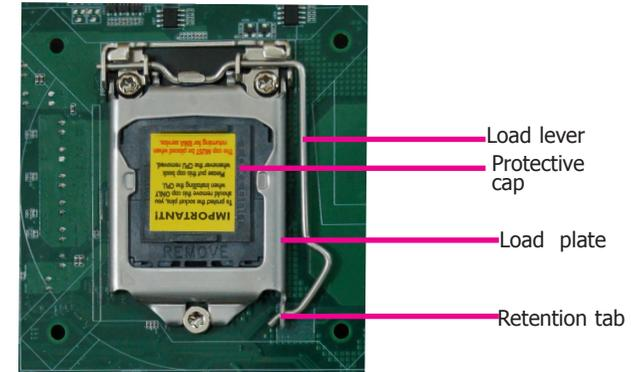
9. Insert the CPU into the socket. The gold triangular mark on the CPU must align with the corner of the CPU socket as shown below. The CPU's notch will at the same time fit into the socket's alignment key.
