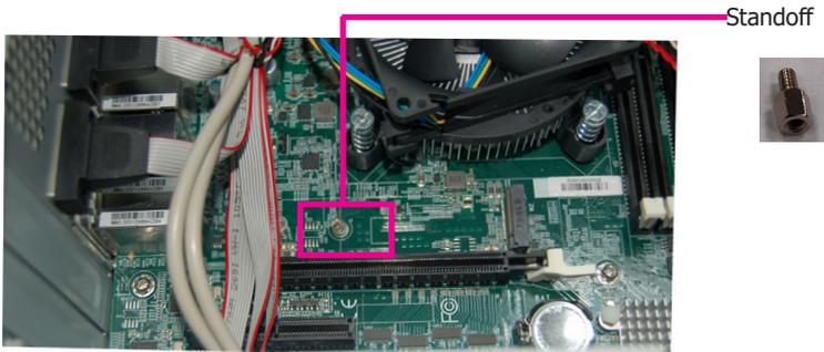
2. Align the notch at the edge of the M.2 card with the key in the connector.
