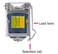
5. Lifting the load lever will at the same time lift the load plate.
