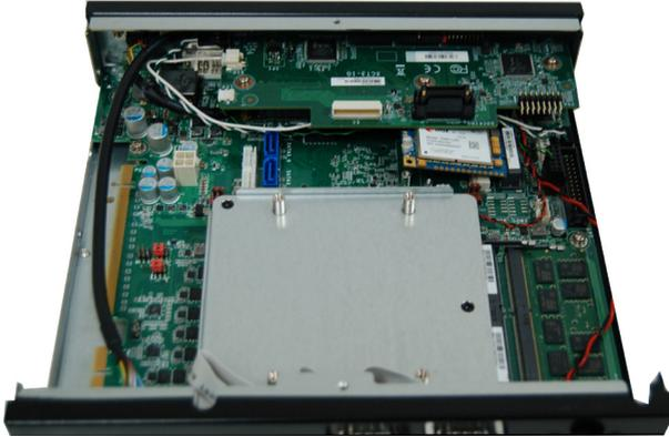
2. Push the Mini PCIe card down and use the provided mounting screw to secure the card on the system board.
