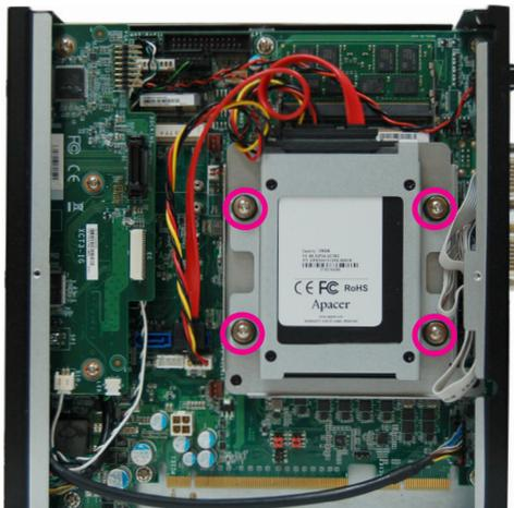
3. Connect the other end of the SATA data/power cable to the SATA data and power connectors on the system board respectively.
