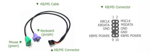
The Keyboard/Mouse connector is used to connect PS/2 keyboard and PS/2 mouse by means of a PS/2 cable.
