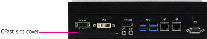
2. Gently insert the CFast card straight with the label on the CFast card facing up until you feel it lock into place. Do not force the card into the slot if the card is not correctly inserted.
