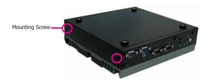
3. Lift the cover upward to open the system.
