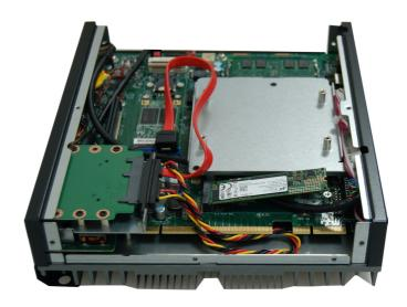
To install an M.2 card, insert the bottom edge of the M.2 card into the connector, and then secure the card to the standoff with the provided mounting screw.
