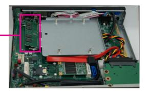
SODIMM module installed into the socket
