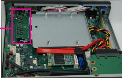
SODIMM module installed into the socket
