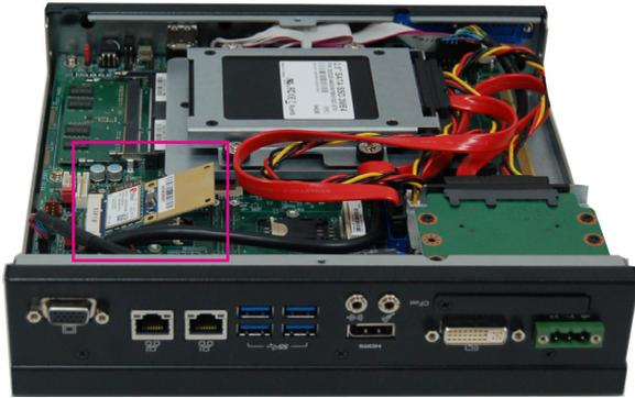
2. Push the Mini PCIe card down and use the provided mounting screws to secure the card on the system board.
