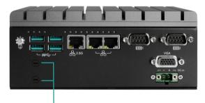
Knockout tabs for Antenna Hole
