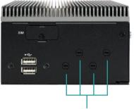
Knockout tabs for Antenna Hole
