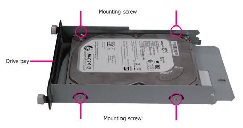
2. Slide the HDD drive tray with the installed hard drive into the optical drive bay and secure the installation with the thumb screws.
