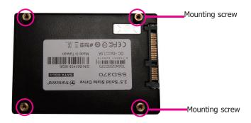
Secure the hard drive to the optical drive tray. Align the standoffs on the HDD with the mounting holes on the optical drive tray. Use 4 mounting screws to install the hard drive onto the optical drive tray.
