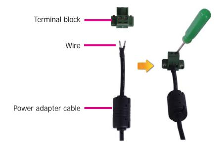
2. Plug the terminal block into the DC-in connector and then tighten the screws to secure the terminal block in place.
