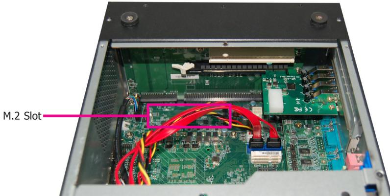
To install an M.2 card, insert the bottom edge of the M.2 card into the connector, and then secure the card to the standoff with the provided mounting screw.
