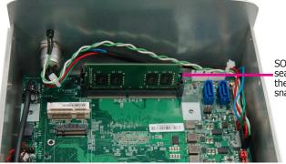
SODIMM is firmly seated in place with the retaining clips snapped behind
