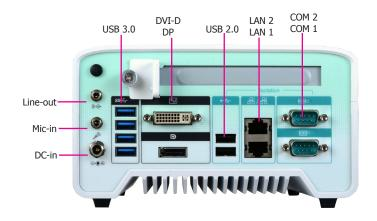
The rear panel I/O consists of the following ports:
