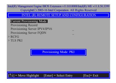
32. In the "Intel(R) Remote Setup And Configuration" menu, select "Provisioning Record" and then press "Enter".
