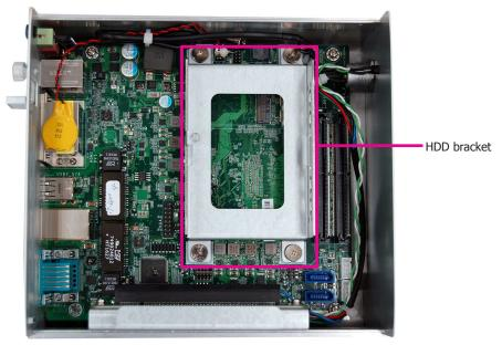
2. Insert the SATA drive into the HDD bracket and secure it in place with the provided screws. Connect the data and power cables to the drive.
