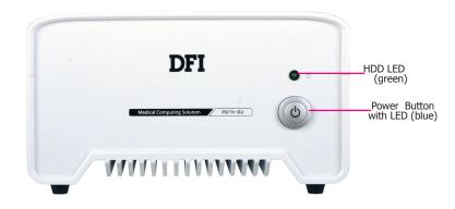
The front panel I/O consists of the following ports:
