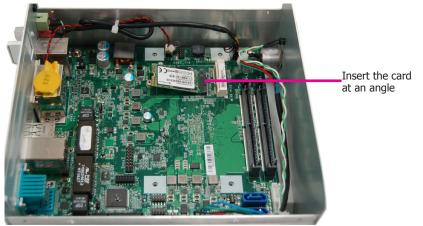
3. Push down on the other end of the M.2 card and secure and card on the mainboard with the provided mounting screw (same size as the Mini PCIe screw).
