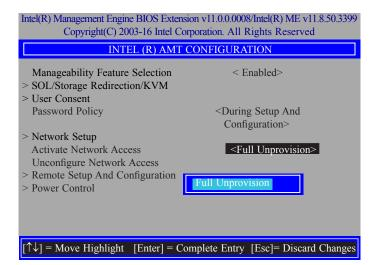
30. In the "Intel(R) AMT Configuration" menu, select "Remote Setup And Configuration" and then press "Enter".
