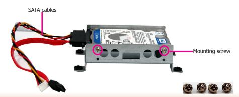
3. Place the SATA drive with the HDD bracket into the system. Align the mounting holes on the HDD bracket with the mounting holes on the mainboard and use the provided screws to secure the drive in place.
