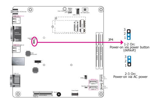
This jumper is used to select the method of powering on the system. If you want the system to power on whenever AC power comes in, set the jumper pins 2 and 3 to "On." If you want to use the power button, set pins 1 and 2 to "On."
