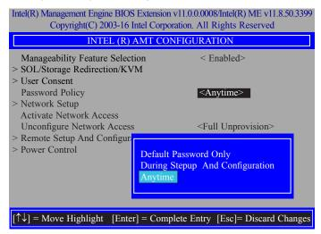
20. In the "Intel(R) AMT Configuration" menu, select "Network Setup" and then press "Enter".
