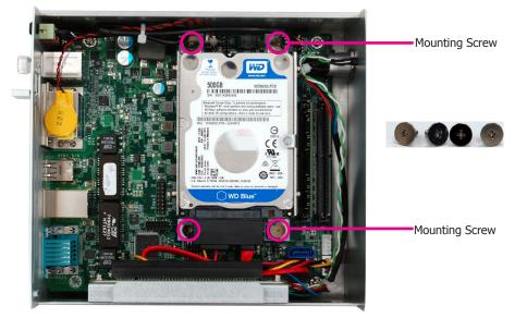
Connect the other end of the SATA data cable and the SATA power cable to the SATA data 4. and SATA power connector on the mainboard respectively.
