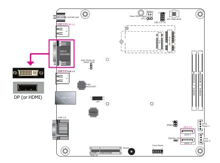
The DVI-D and DP (DisplayPorts) are used to connect an LCD monitor.
