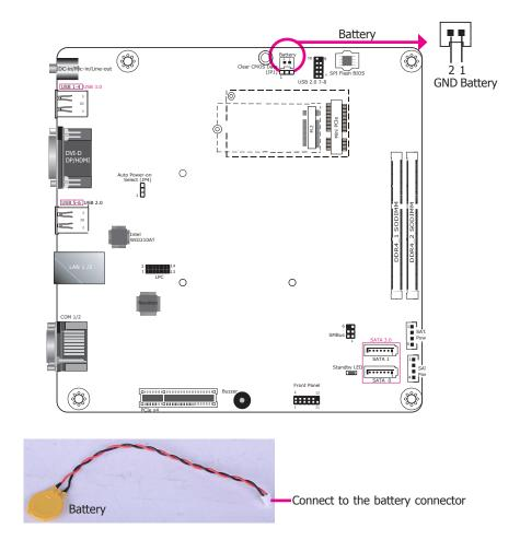
The lithium ion battery powers the real-time clock and CMOS memory. It is an auxiliary source of power when the main power is shut off.
