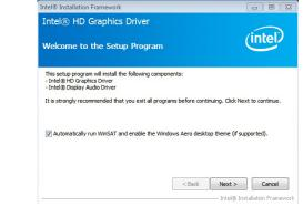
By default, the "Automatically run WinSAT and enable the Windows Aero desktop theme" is enabled. With this enabled, after installing the graphics driver and the system rebooted, the screen will turn blank for 1 to 2 minutes (while WinSAT is running) before the Windows 7/Windows 8.1/Windows 10 desktop appears. The "blank screen" period is the time Windows is testing the graphics performance.
