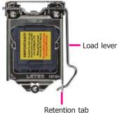
The CPU socket must not come in contact with anything other than the CPU. Avoid unnecessary exposure. Remove the protective cap only when you are about to install
