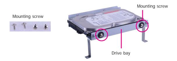
4. Place the drive bay back in the chassis and install the drive bay using the mounting screws you removed in step 1.
