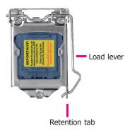
5. Lifting the load lever will at the same time lift the load plate.
