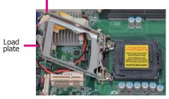
Remove the protective cap from the CPU socket. The cap is used to protect the CPU socket against dust and harmful particles. Remove the protective cap only when you are about to install the CPU.
