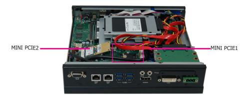
2. Push the Mini PCIe card down and use the provided mounting screws to secure the card on the system board.
