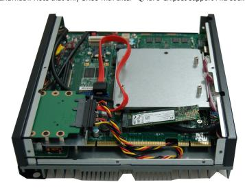
To install an M.2 card, insert the bottom edge of the M.2 card into the connector, and then secure the card to the standoff with the provided mounting screw.
