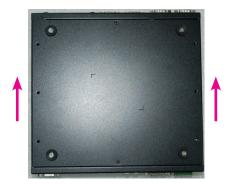
5. The SODIMM sockets, Mini PCIe and M.2 slots and SATA drive bay can be easily accessed after the chassis cover is removed.
