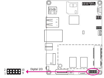
The Digital I/O connector supports 8-bit digital input/output signals to provide powering-on function of the connected devices.
