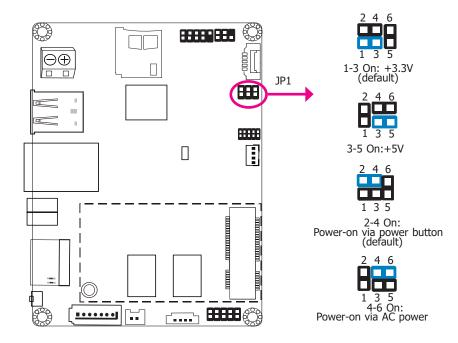
JP1 is used to select the method of powering on the system. If you want the system to power on whenever AC power comes in, set JP1 pins 4 and 6 to On. If you want to use the power button, set pins 2 and 4 to On.
