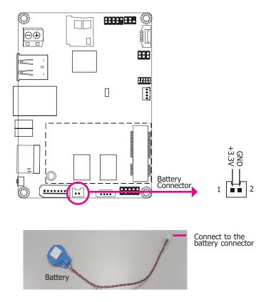
The lithium ion battery powers the real-time clock. It is an auxiliary source of power when the main power is shut off.
