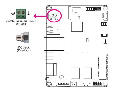
This 2-pin terminal block (for Quad) or DC jack (for DualLite) is considered a low power solution. Connect a DC power cord to this terminal block or jack. Using a voltage more than the recommended range may fail to boot the system or cause damage to the system board.
