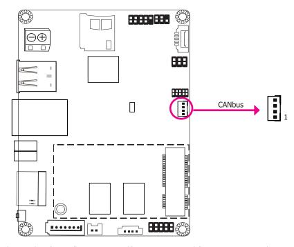
The CAN bus (Controller Area Network) connector is used for interconnecting electronic control units (ECUs).
