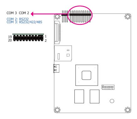
COM 2 is fixed at RS232 whereas COM 3 can be selected among RS232, RS422 and RS485. RS485 communication supports auto flow control.
