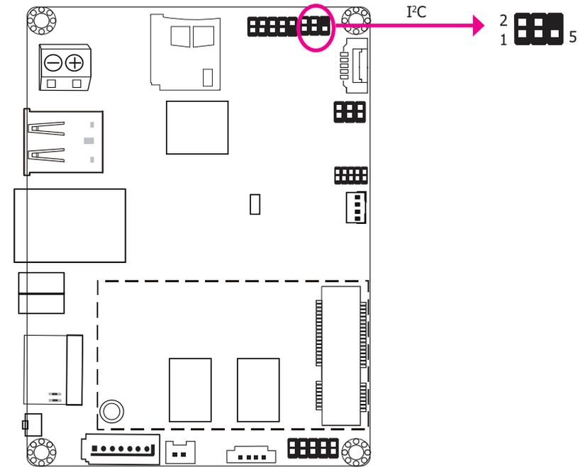
The I<sup>2</sup>C connector is used to monitor or communicate with system components.
