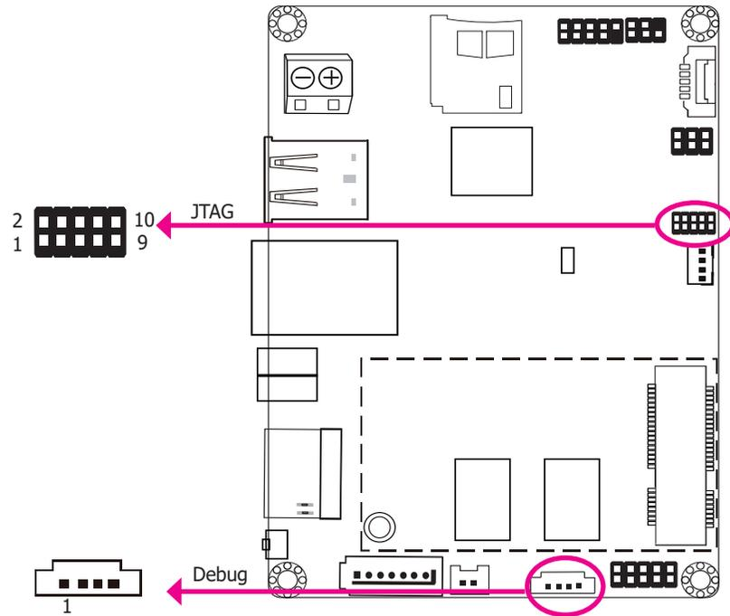
The JTAG and debug connectors are used for debugging purposes.
