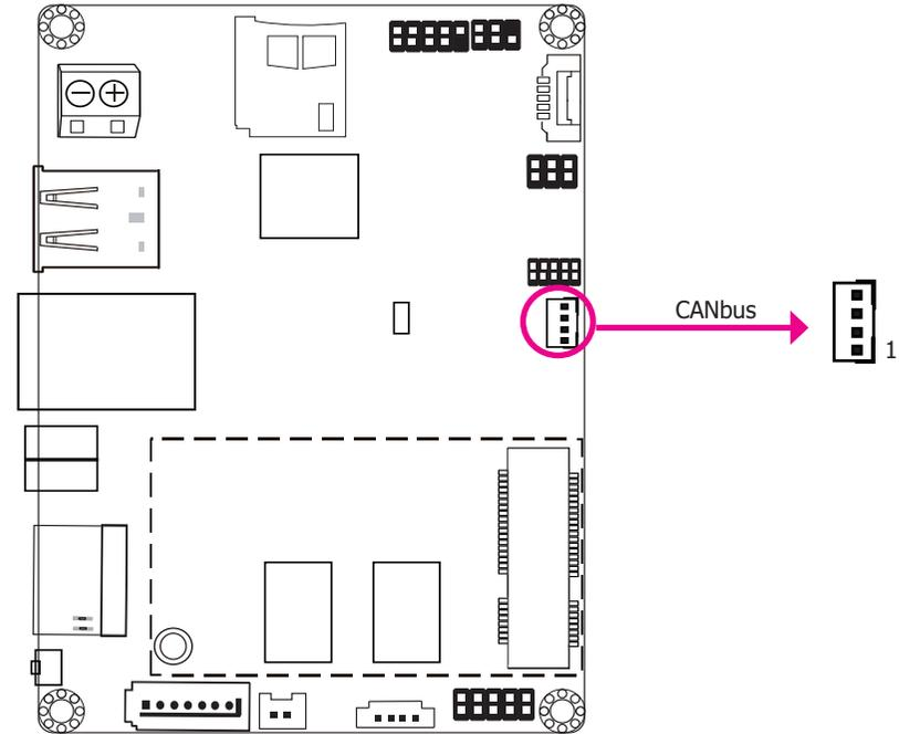
The CAN bus (Controller Area Network) connector is used for interconnecting electronic control units (ECUs).
