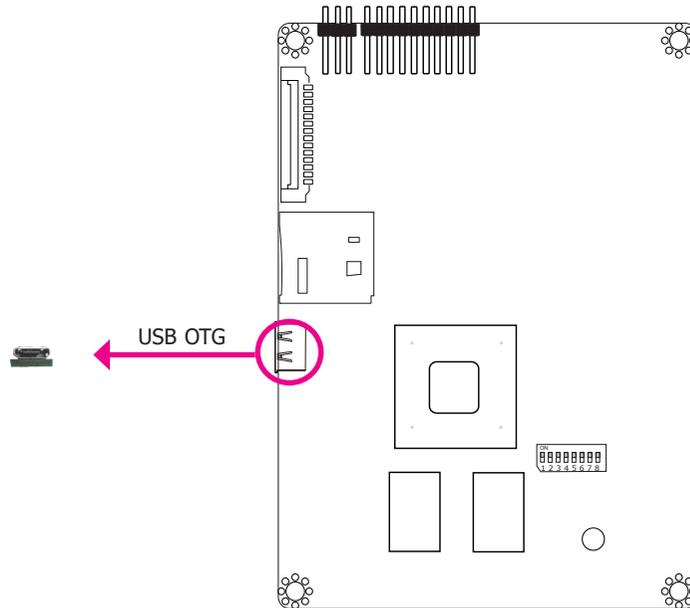
The USB OTG (USB 2.0) port is used for USB communication.
