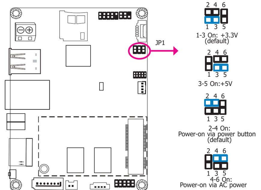
JP1 is used to select the method of powering on the system. If you want the system to power on whenever AC power comes in, set JP1 pins 4 and 6 to On. If you want to use the power button, set pins 2 and 4 to On. When using the JP1 "Power On" feature to power the system back on after a power failure occurs, the system may not power on if the power lost is resumed within 5 seconds (power flicker).
