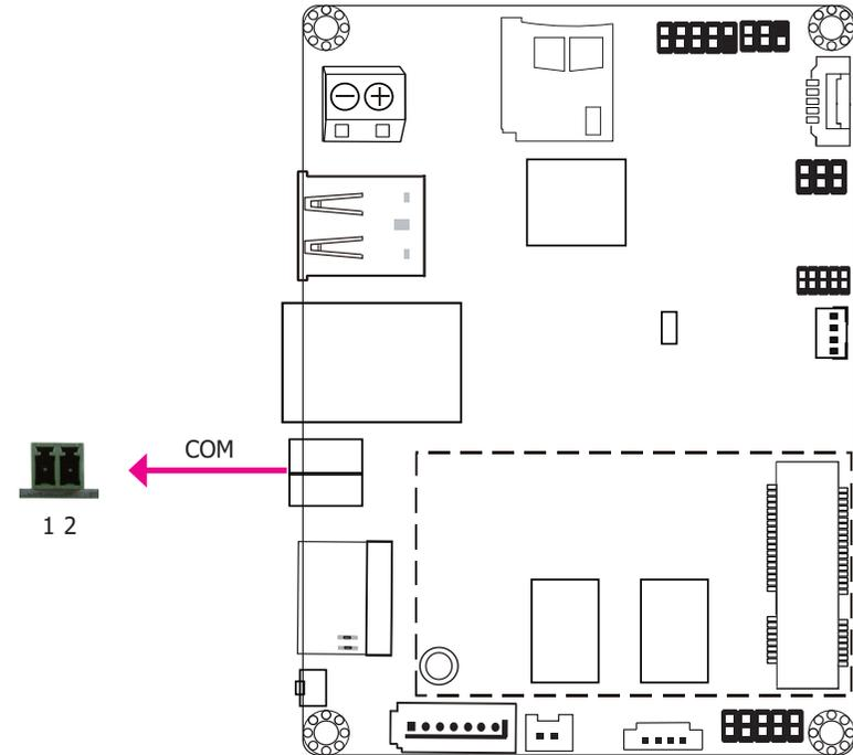
The serial port provides 2-wire RS485 communication with support of auto flow control.
