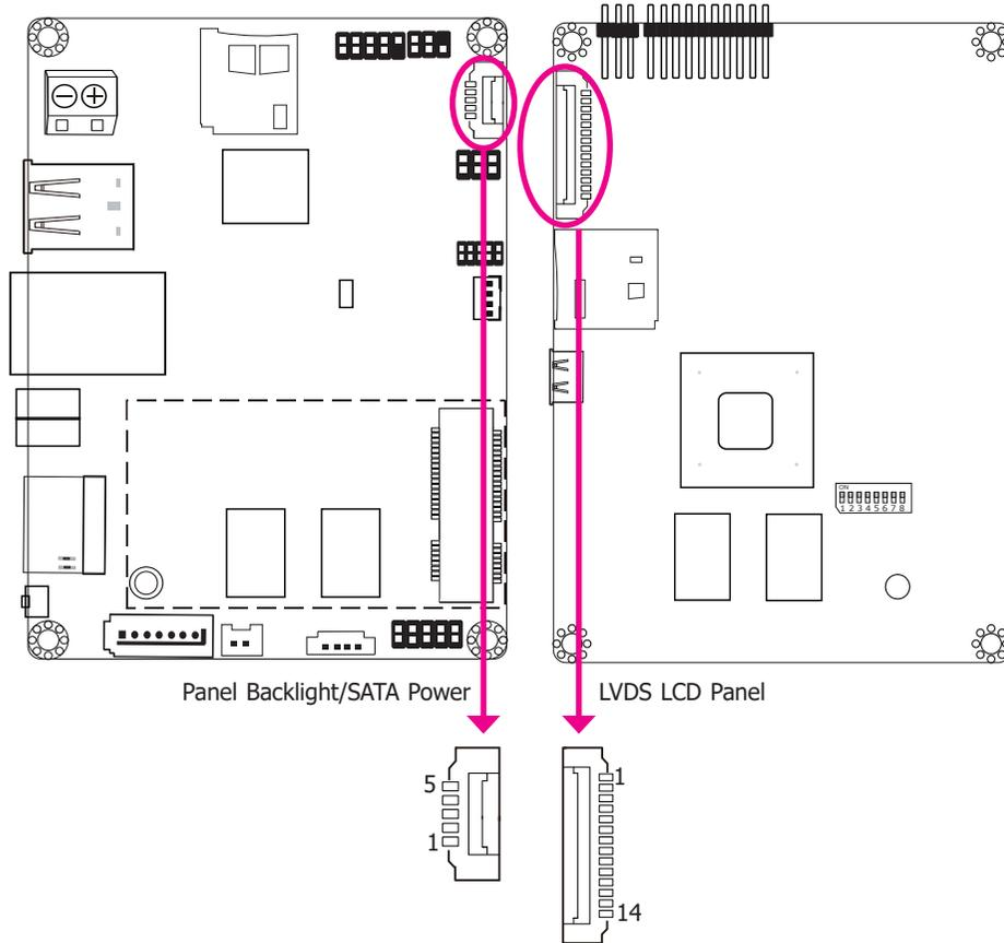
The system board allows you to connect a LCD Display Panel by means of the LVDS LCD panel connector and the Panel Backlight/SATA power connector. These connectors transmit video signals and power from the system board to the LCD Display Panel. Panel Backlight/SATA power connector also supplies power to the SATA drive. Connect one end of the provided power cable to the SATA power connector and the other end to your storage device.
