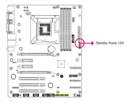
This LED will lit red when the system is in the standby mode. It indicates that there is power on the system board. Power-off the PC and then unplug the power cord prior to installing any devices. Failure to do so will cause severe damage to the motherboard and components.
