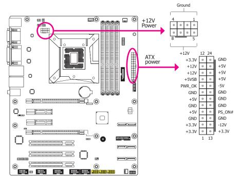
Use a power supply that complies with the ATX12V Power Supply Design Guide Version 1.1. An ATX12V power supply unit has a standard 24-pin ATX main power connector that must be inserted into the 24-pin connector. The 8-pin +12V power connector enables the delivery of more +12VDC current to the processor's Voltage Regulator Module (VRM).
