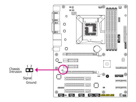
The board supports the chassis intrusion detection function. Connect the chassis intrusion sensor cable from the chassis to this connector. When the system's power is on and a chassis intrusion occurred, an alarm will sound. When the system's power is off and a chassis intrusion occurred, the alarm will sound only when the system restarts.
