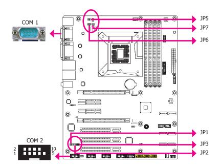
JP5 (for COM1) and JP1 (for COM2) are used to configure the COM ports to RS232, RS422 (Full Duplex) or RS485. The pin functions of the COM ports will vary according to the jumper's setting.
