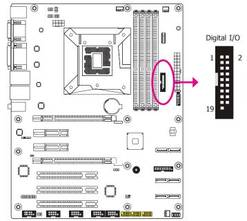
The 8-bit Digital I/O connector provides powering-on function to external devices that are connected to these connectors.
