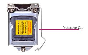
4. Unlock the socket by pushing the load lever down, moving it sideways until it is released from the retention tab; then lift the load lever up.
