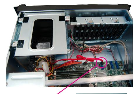
3. Connect the SATA data cable and the SATA power cable to the connectors on the SATA drive.
