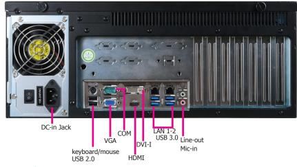
DC-in jack Used to plug a power adapter.
