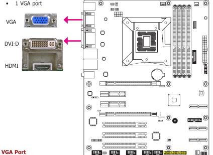
The VGA port is used for connecting a VGA monitor. Connect the monitor's 15-pin D-shell cable connector to the VGA port. After you plug the monitor's cable connector into the VGA port, gently tighten the cable screws to hold the connector in place.
