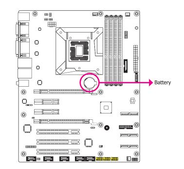
The lithium ion battery powers the real-time clock and CMOS memory. It is an auxiliary source of power when the main power is shut off.
