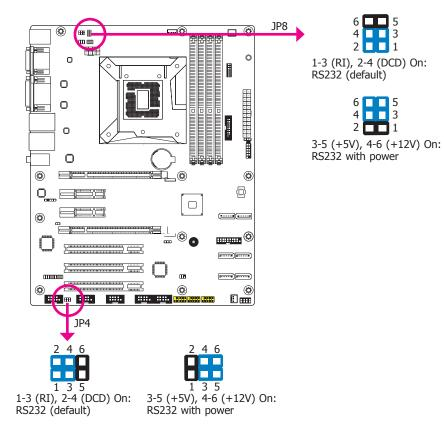
JP8 (for COM 1) and JP4 (for COM 2) are used to configure Serial COM ports to pure RS232 or RS232 with power. The pin functions of COM 1 and COM 2 will vary according to JP8's and JP4's setting respectively.
