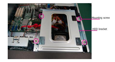
2. Align the mounting holes of the SATA drive with the mounting holes on the HDD brackets and then use the mounting screws to secure the drive in place.
