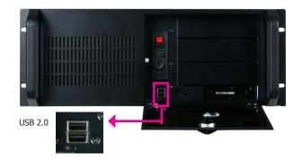
The USB device allows data exchange between your computer and a wide range of simultaneously accessible external Plug and Play peripherals.
