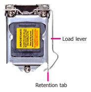
5. Lift the load lever to lift the load plate. Lift the load lever up to the angle shown on the photo.
