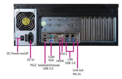
The rear panel I/O consists of the following ports:
