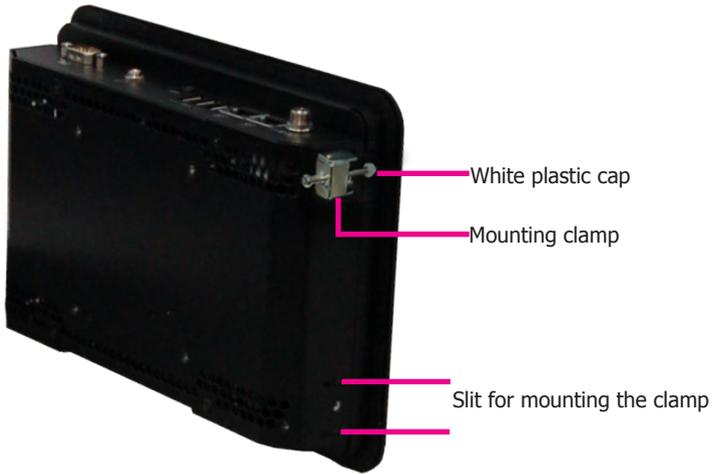
5. Position the mounting clamps along the rear edges of the Panel PC and insert them into the slits around the Panel PC.
