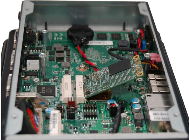
2. Push the Mini PCIe card down and use the provided mounting screws to secure the card on the system board.
