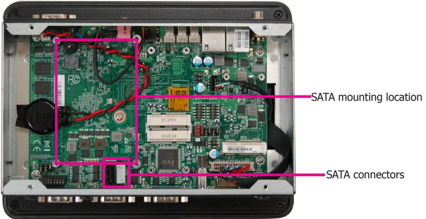
2. Align the mounting holes of the SATA HDD with the mounting holes on the HDD drive bay and use the provided mounting screws to attach the SATA HDD to the drive bay.
