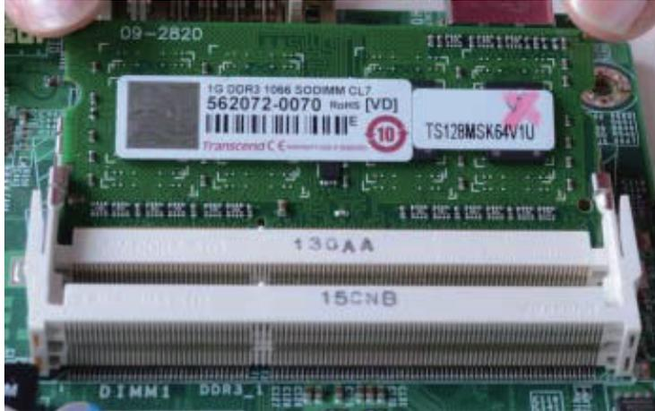
6. Push down the module until the clips at each end of the socket lock into position. You will hear a distinctive "click", indicating the module is correctly locked into position.
