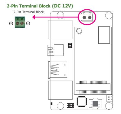
This 2-pin terminal block is considered a low power solution. Connect a power adaptor and 2-pole terminal to DC jack cable to this terminal block. Using a voltage more than the recommended range may fail to boot the system or cause damage to the system board.
