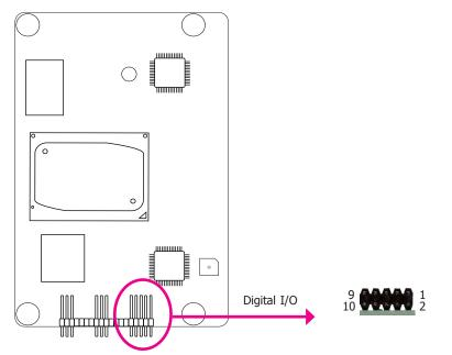
The Digital I/O connector supports 8-bit digital input/output signals to provide the ability of monitoring and controlling the states of the connected external devices.
