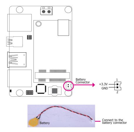
The lithium ion battery powers the real-time clock and CMOS memory. It is an auxiliary source of power when the main power is shut off.
