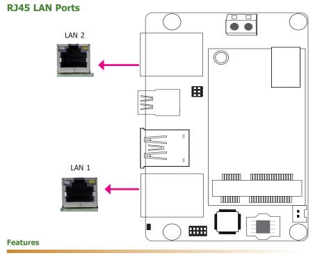
• 2 Intel<sup>®</sup> I210AT PCI Express Gigabit Ethernet controllers or 2 optional Intel<sup>®</sup> I210IT PCI Express Gigabit Ethernet controllers
