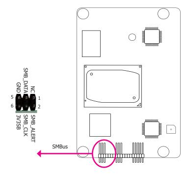
The System Management Bus (SMBus) connector is used to connect SMBus devices. It is a multiple device bus that allows multiple chips to connect to the same bus and enable each one to act as a master by initiating data transfer.
