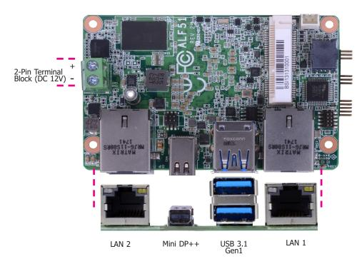
The rear panel I/O consists of the following ports:
