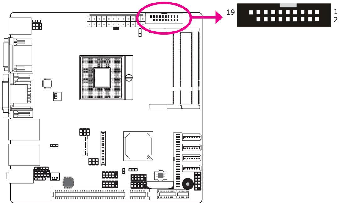
The Digital I/O connector provides powering-on function to an external device that is connected to this connector.
