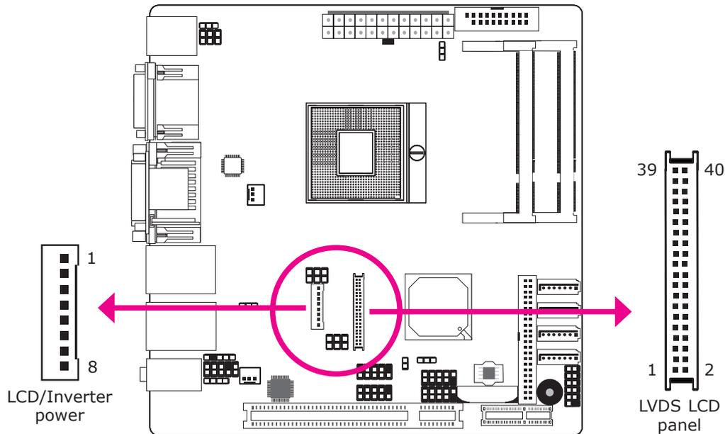
The system board allows you to connect a LCD Display Panel by means of the LVDS LCD panel connector and the LCD/Inverter power connector. These connectors transmit video signals and power from the system board to the LCD Display Panel.
