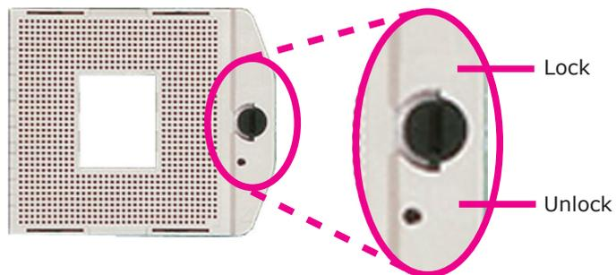
5. Position the CPU above the socket. The gold triangular mark on the CPU must align with pin 1 of the CPU socket.
