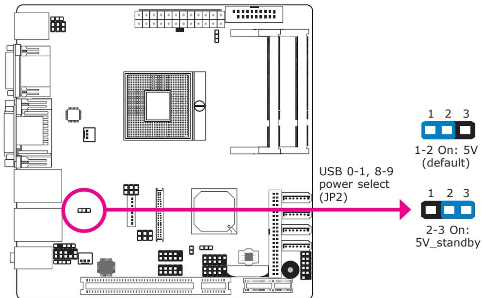
JP2 (for USB 0-1 and USB 8-9) is used to select the power of the USB ports. Selecting 5V\_standby will allow you to use a USB device to wake up the system.
