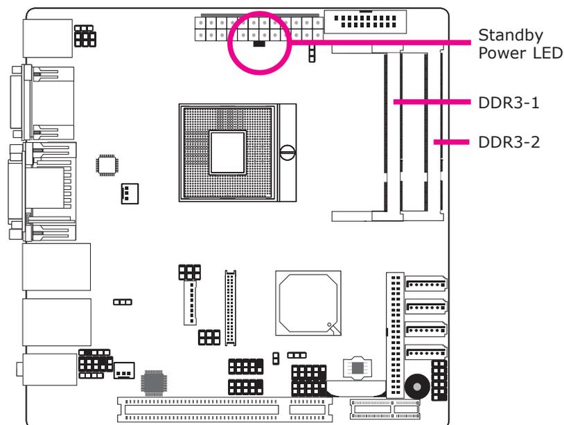
The system board is equipped with two 204-pin SODIMM sockets that support DDR3 memory modules.
