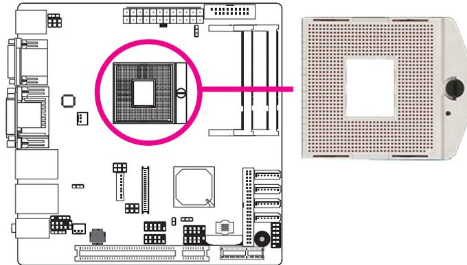
4. Make sure the screw is in its unlock position. If it's not, use a screwdriver to turn the screw to its unlock position.
