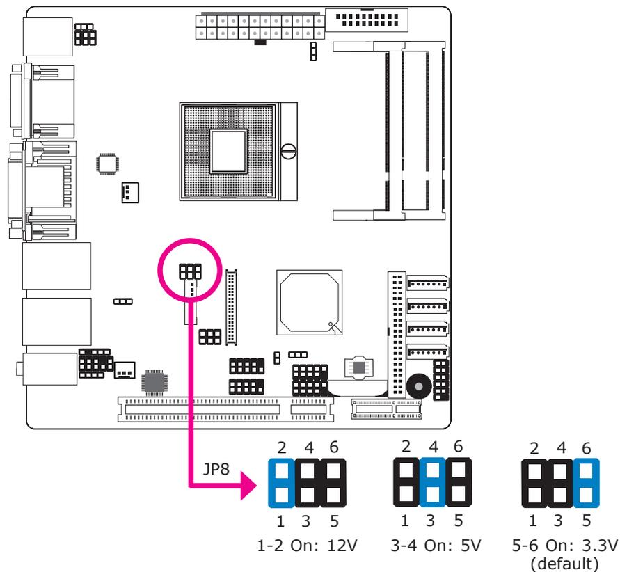
JP8 is used to select the power supplied to the LCD panel.
