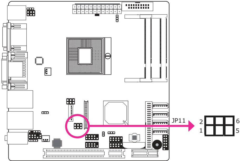
JP11 is used to configure COM 3 to RS232 or RS485.
