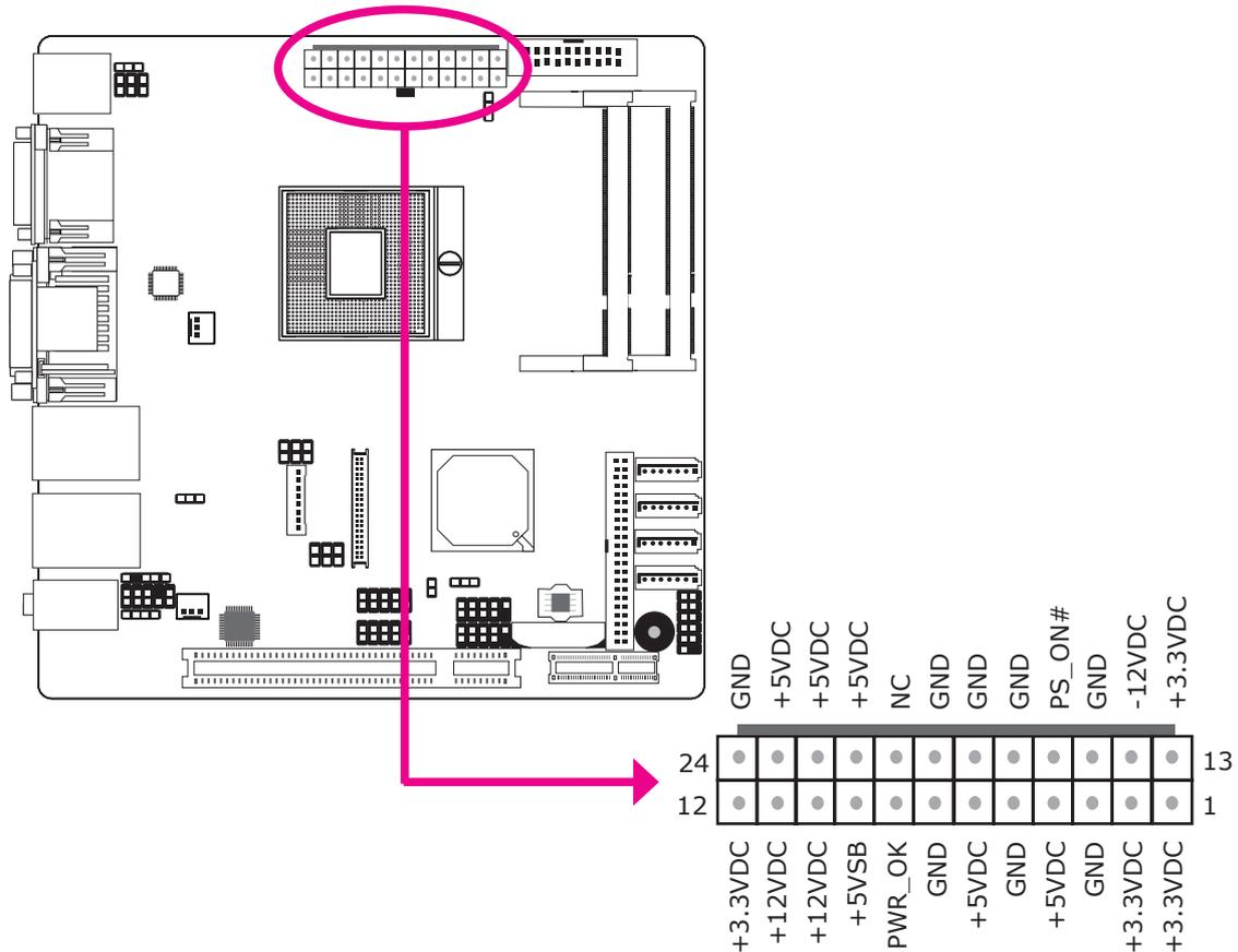
Connect a 24-pin ATX main power connector from the power supply unit to the 24-pin power connector. The connector from the power supply unit is designed to fit the 24-pin connector in only one orientation. Make sure to find the proper orientation before plugging the connector.
