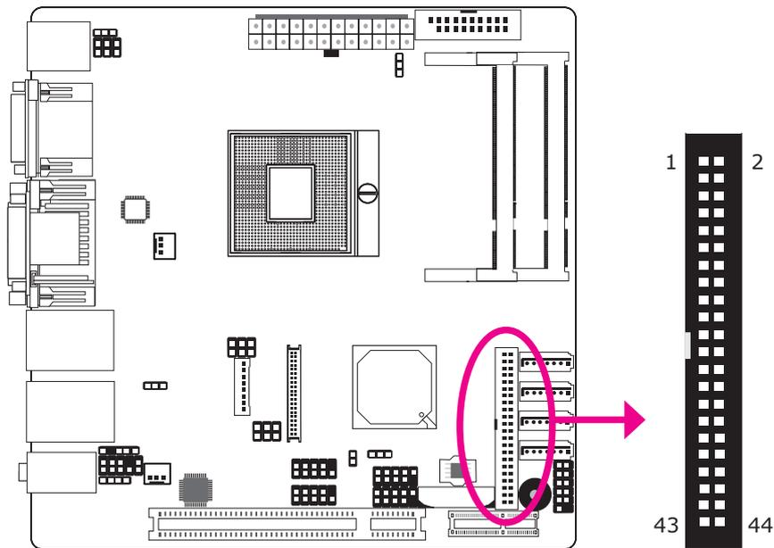
The IDE connector is used to connect hard drives. The connector on the IDE cable can be inserted into this connector only if pin 1 of the cable is aligned with pin 1 of this connector.
