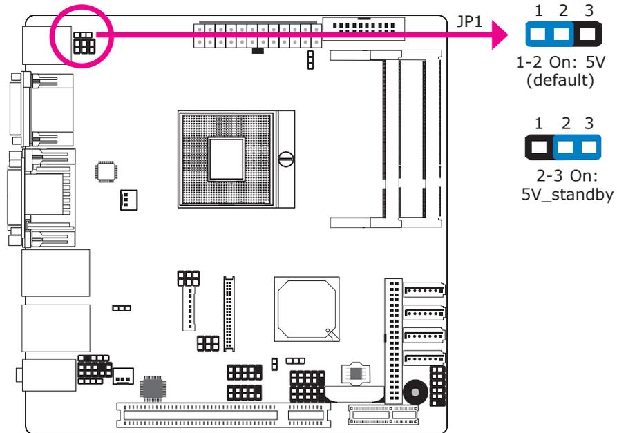
JP1 is used to select the power of the PS/2 keyboard/mouse port. Selecting 5V\_standby will allow you to use the PS/2 keyboard or PS/2 mouse to wake up the system.
