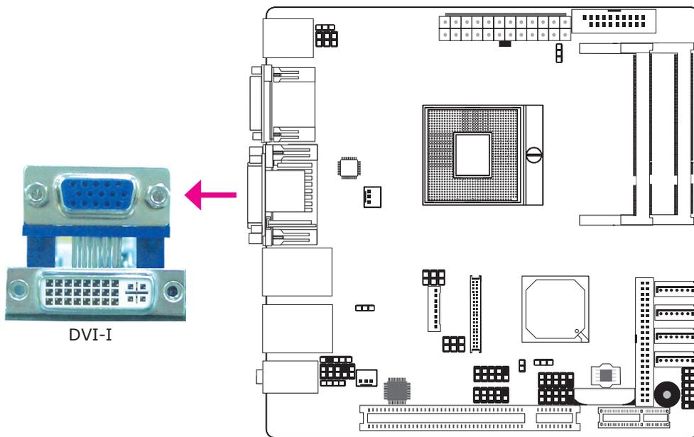
The DVI-I port is used to connect an LCD monitor. This port supports DVI-D signal only.
