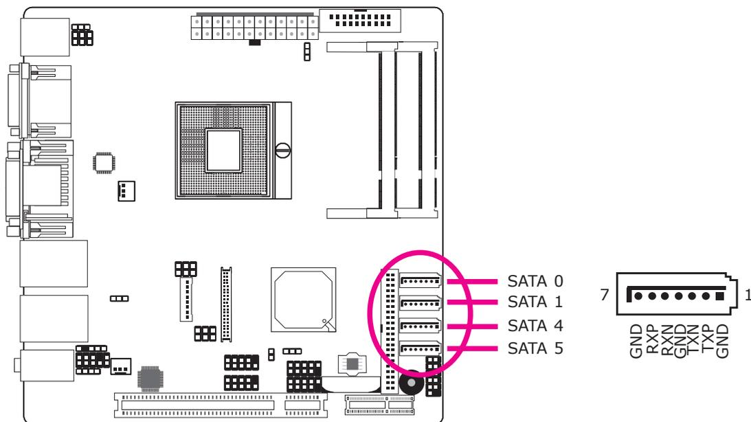
The Serial ATA connectors are used to connect Serial ATA devices. Connect one end of the Serial ATA cable to a SATA connector and the other end to your Serial ATA device.
