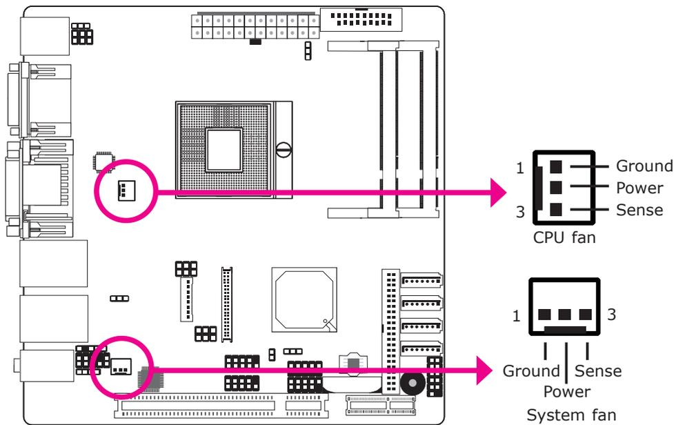
The fan connectors are used to connect cooling fans. The cooling fans will provide adequate airflow throughout the chassis to prevent overheating the CPU and system board components.
