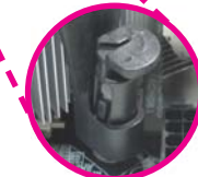
"Unlocked" position of push-pin
