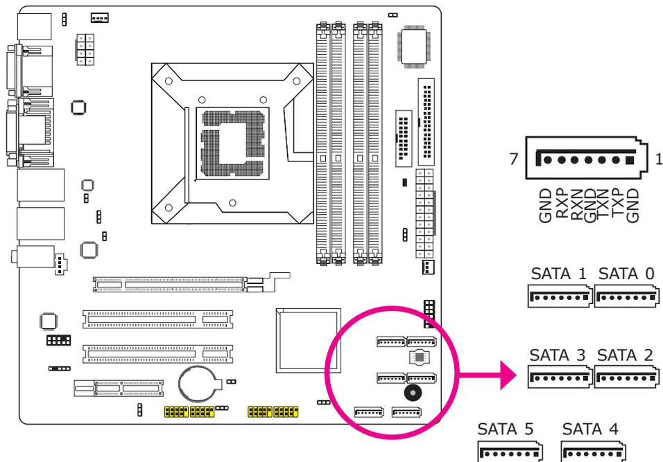
The Serial ATA ports are used to connect Serial ATA devices. Connect one end of the Serial ATA cable to a SATA port and the other end to your Serial ATA device.
