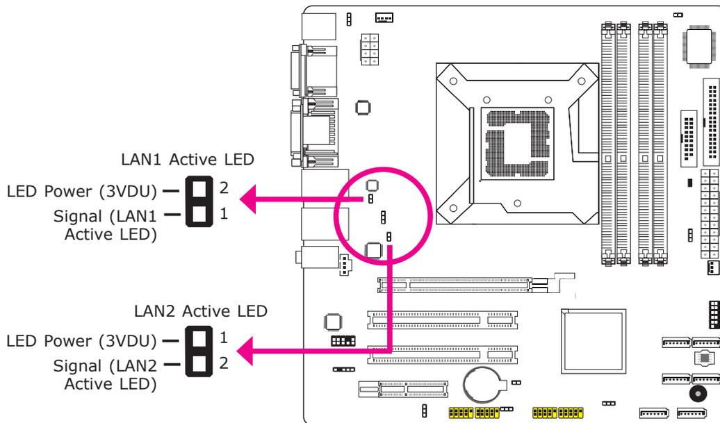
The LAN Active LED connectors are used to connect to the LAN LEDs that are usually located at the front panel of the chassis.
