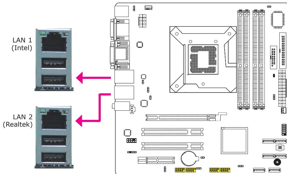
The LAN ports allow the system board to connect to a local area network by means of a network hub.
