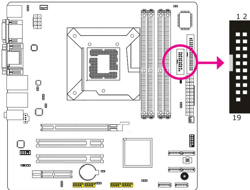
The Digital I/O connector provides powering-on function to an external device that is connected to this connector.
