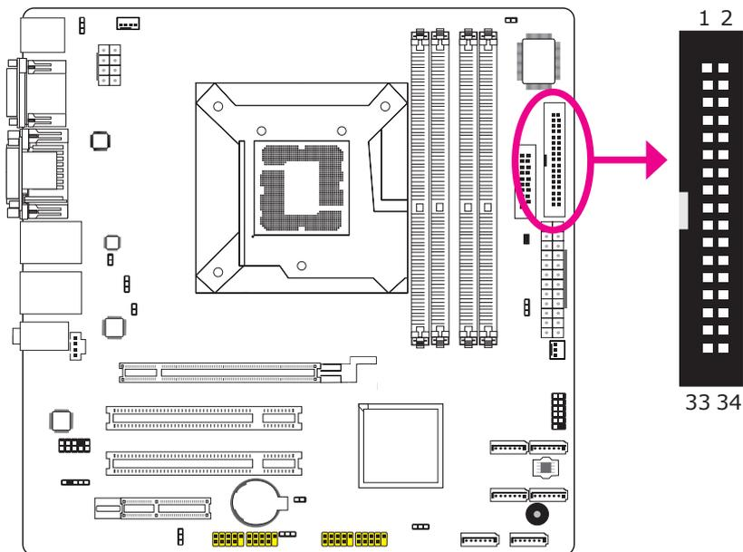
The FDD connector supports a standard floppy disk drive. The floppy cable can be inserted into this connector only if pin 1 of the cable is aligned with pin 1 of this connector.
