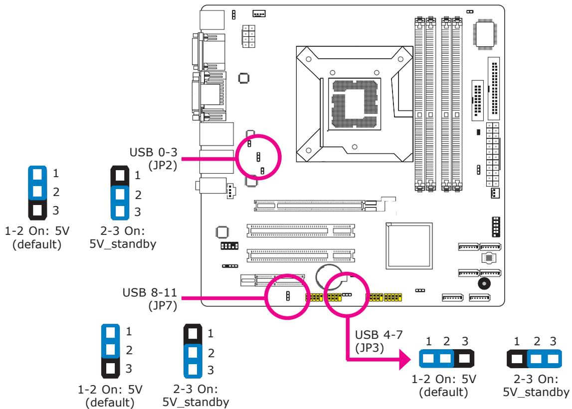
These jumpers are used to select the power of the USB ports. Selecting 5V\_standby will allow you to use a USB device to wake up the system.
