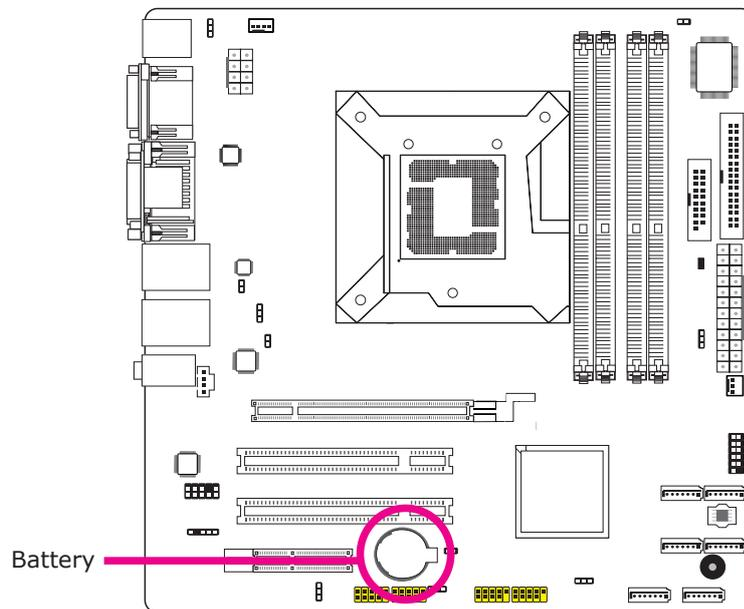
The lithium ion battery powers the real-time clock and CMOS memory. It is an auxiliary source of power when the main power is shut off.
