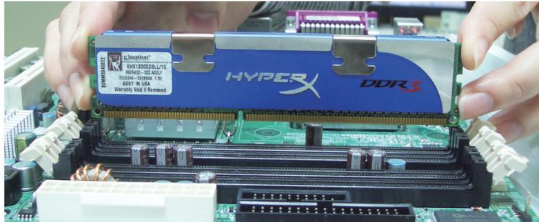
7. Seat the module vertically, pressing it down firmly until it is completely seated in the socket.
