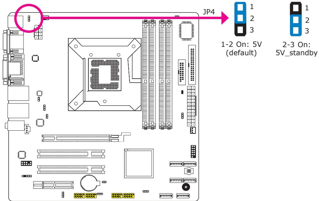
JP4 is used to select the power of the PS/2 keyboard/mouse port. Selecting 5V\_standby will allow you to use a PS/2 keyboard or PS/2 mouse to wake up the system.
