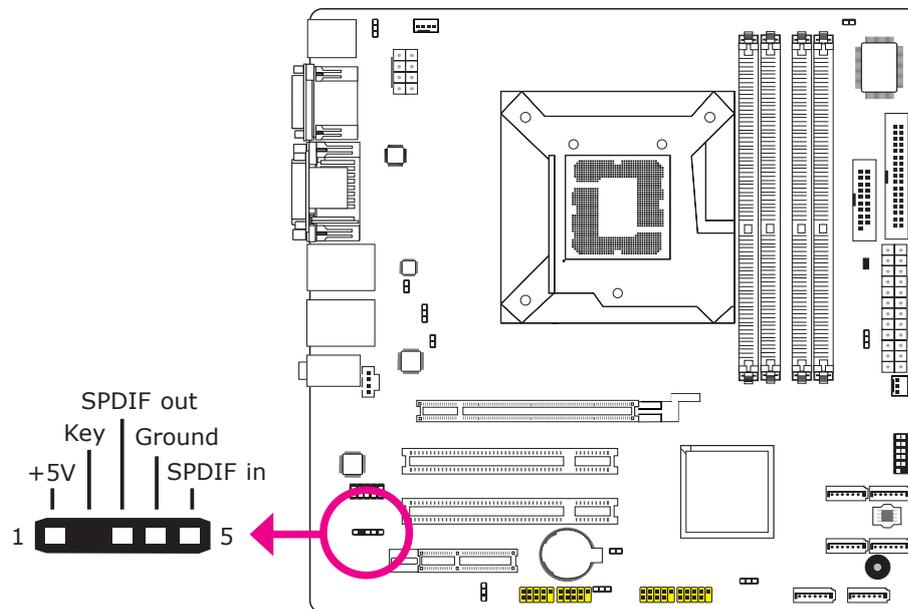
The S/PDIF connector is used to connect an external S/PDIF port. Your S/PDIF port may be mounted on a card-edge bracket. Install the card-edge bracket to an available slot at the rear of the system chassis then connect the audio cable to the S/PDIF connector. Make sure pin 1 of the audio cable is aligned with pin 1 of the S/PDIF connector.
