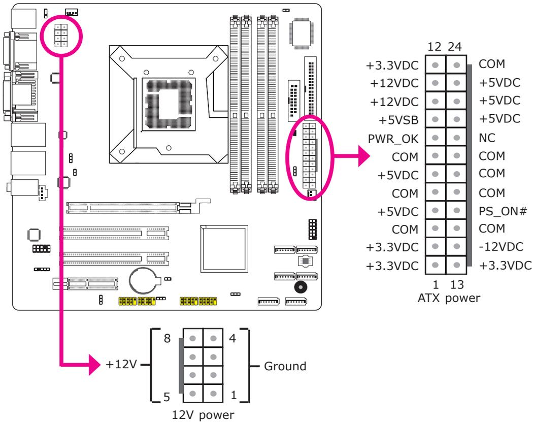
Use a power supply that complies with the ATX12V Power Supply Design Guide Version 2.0. An ATX12V power supply unit has a standard 24-pin ATX main power connector that must be inserted into the 24-pin connector. The 8-pin +12V power connector enables the delivery of more +12VDC current to the processor's Voltage Regulator Module (VRM).
