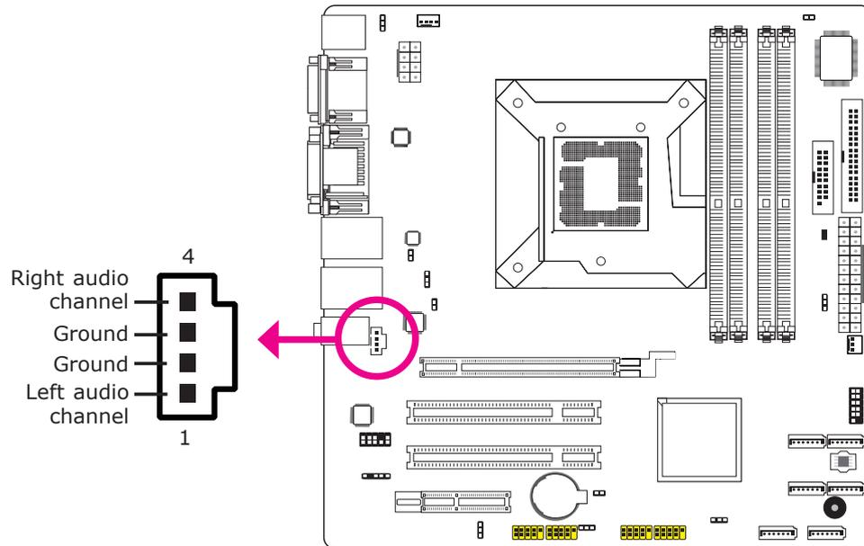
The CD-in connector is used to receive audio from a CD-ROM drive, TV tuner or MPEG card.
