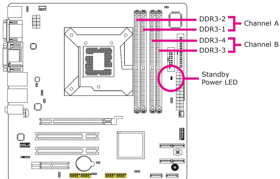
The four DIMM sockets are divided into 2 channels:
