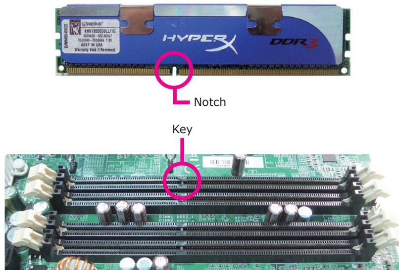
6. Grasping the module by its edges, position the module above the socket with the “notch” in the module aligned with the “key” on the socket. The keying mechanism ensures the module can be plugged into the socket in only one way.
