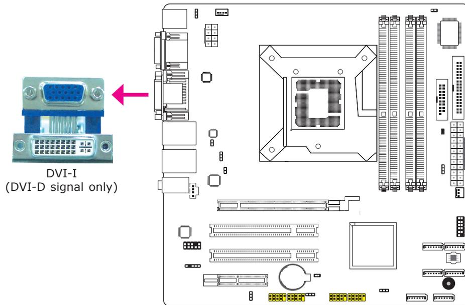
The DVI-I port is used to connect an LCD monitor. This port supports DVI-D signal only.
