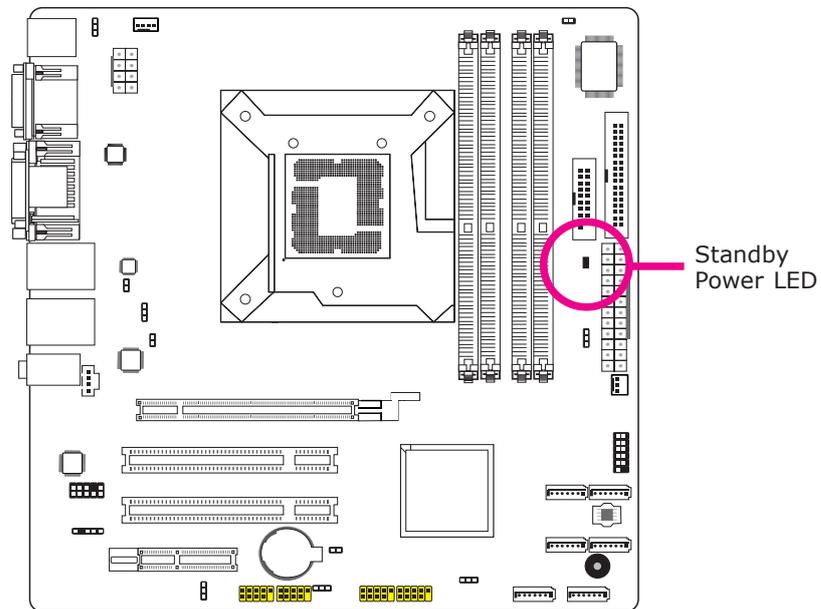
This LED will lit red when the system is in the standby mode. It indicates that there is power on the system board. Power-off the PC then unplug the power cord prior to installing any devices. Failure to do so will cause severe damage to the motherboard and components.
