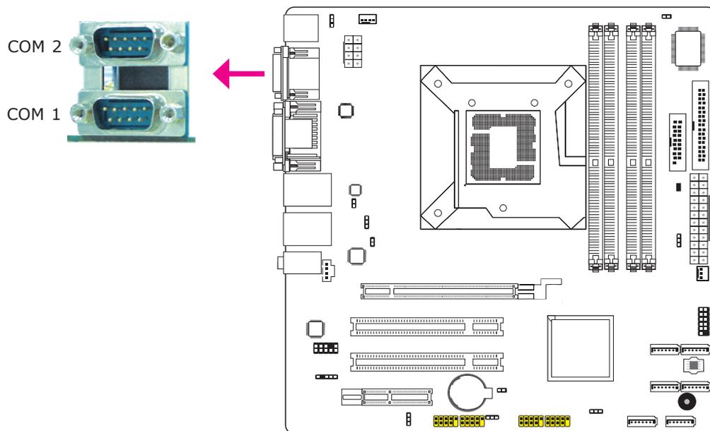
The serial ports are RS232 asynchronous communication ports with 16C550A-compatible UARTs that can be used with modems, serial printers, remote display terminals, and other serial devices.
