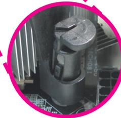
"Unlocked" position of push-pin
