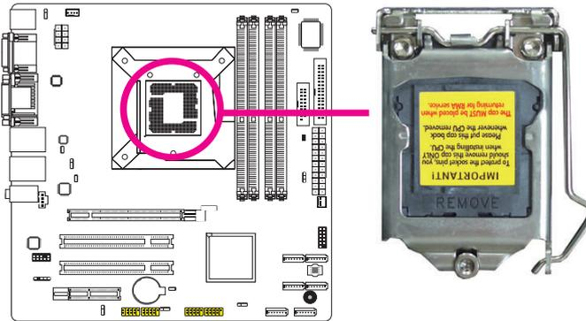
4. Unlock the socket by pushing the load lever down, moving it sideways until it is released from the retention tab; then lift the load lever up.
