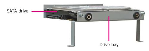
4. Use the provided mounting screws to secure the SATA drive onto the drive bay.
