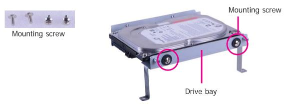
5. Place the drive bay into the chassis. Secure the drive bay with the mounting screws you removed in step 1.
