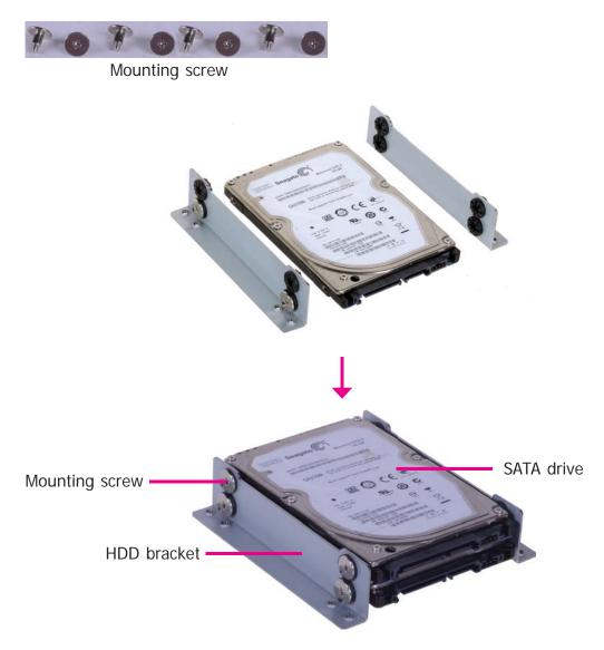
4. Turn to the other side of the drive bay. Use the provided mounting screws from step 2 to secure the SATA drive bay assembly onto the drive bay.
