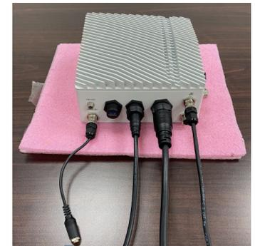
This is a standard power converter cable after assembly; customer can either use our power converter cable or a customized cable to directly connect ECX700 with their power adaptor
