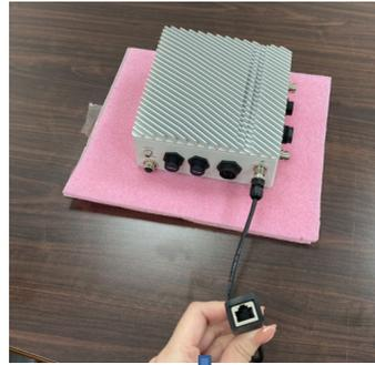
This is a standard LAN converter cable after assembly; customer can either use our converter cable or a customized cable to directly connect ECX700 with their devices
